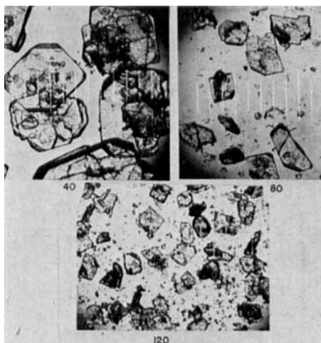
Fig. 1.—Various fractions of tripeleminamine HCl. The linear distance between each white scale line is 100 microns.
